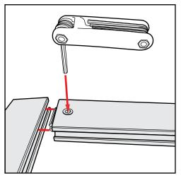
**Extrusion & Lock Connection**
