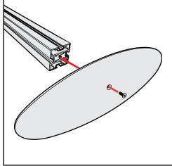
Base Plate & Extrusion Connection
