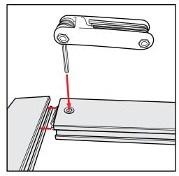
**Extrusion & Lock Connection**
