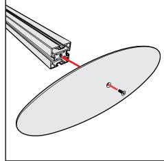
Base Plate & Extrusion Connection
