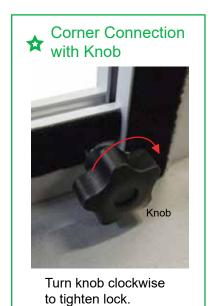
Do not over tighten Knobs
