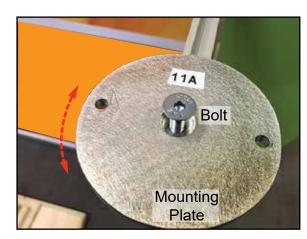
3) Place mounting plate onto [10] then tighten bolt, part way, allowing some rotation for final positioning.
